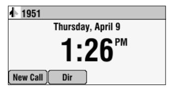
The shared line icon changes to a moving icon, and the LEDs glow a steady red when the line is in use remotely.
